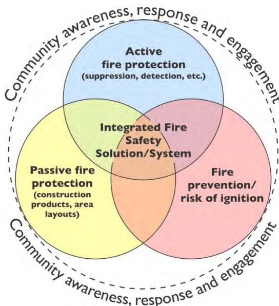
Figure 1-4: Framework for addressing informal settlement fire safety (adapted from 9)
