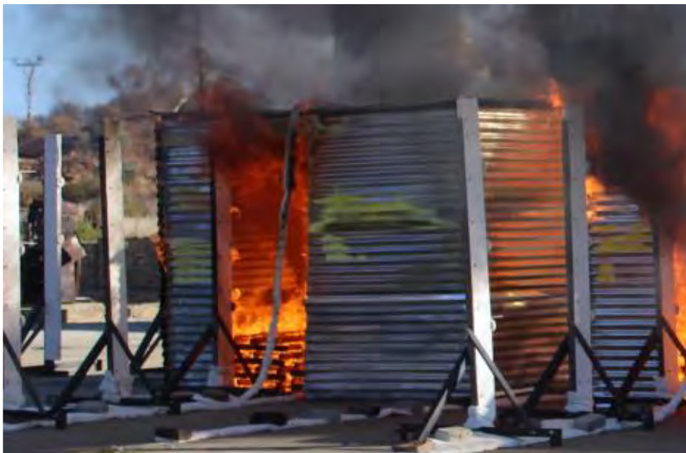
Figure 6-12: Example of an informal dwelling during a fire, with the galvanising (zinc) melting and starting to run down the side (occurring at position of green-yellow colour). Galvanised sheeting heats up only marginally slower than normal sheeting, and should not be regarded as fire-rated.
