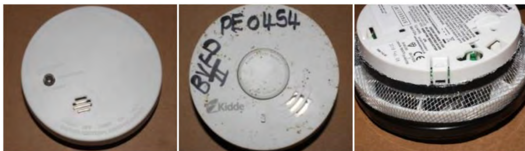
Figure 6-9: (Left) Example of an ionisation smoke alarm, (Middle) Example of a photoelectric smoke alarm with a dust button that was used in a project, but experienced problems probably due to bug infestation (the small brown marks on the device are insect faeces), and (Right) ongoing testing through investigating how to prevent insects from getting into devices by installing items such as a steel mesh.
